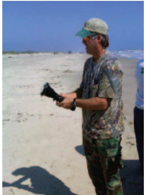
Figure 6. Super Talon net gun and operator. This method of capture was far less of a disturbance than the Coda Netgun when discharged, but it was underpowered, resulting in a reduced effective range.
