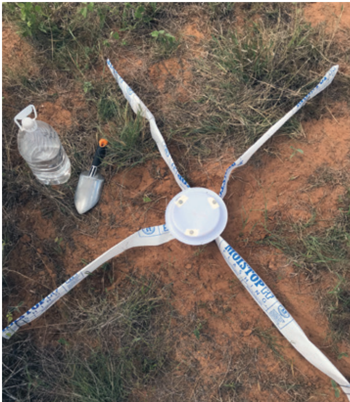
Figure 4. Pitfall trap design with X-shaped guidance barriers used on the San Antonio Viejo Ranch, Jim Hogg and Starr counties, TX, USA in July-August 2019.
